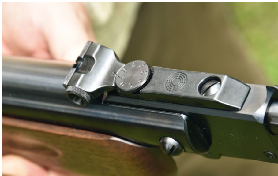
The barrels are now fitted into the breech block with a locking nut
