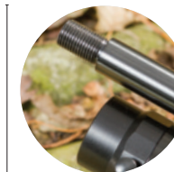
The barrel is screw-cut with a standard 1/2in UNF thread, but the thread is far longer than usual, making for a more sturdy connection with your moderator
