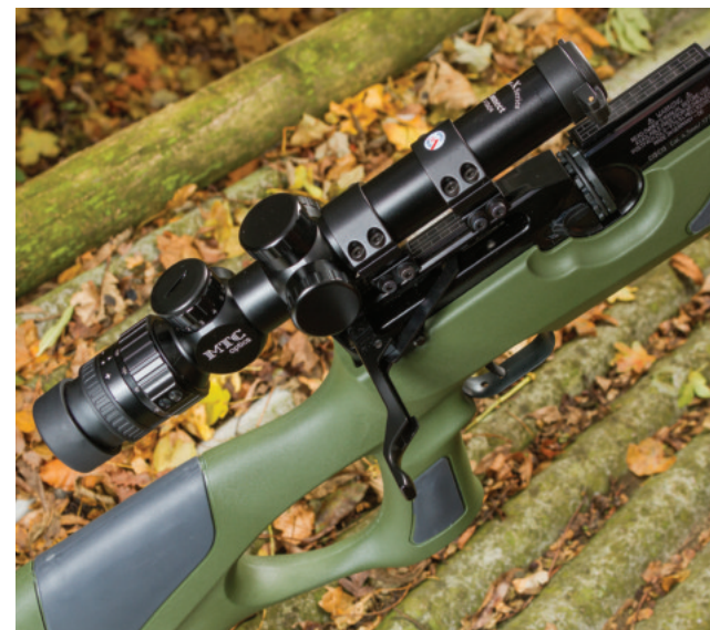
The cocking lever is slick to use and lays almost flush with the action when not in use, meaning it's less likely to snag on clothing
