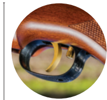
The trigger weight adjustment screw is located behind the blade. It can be adjusted with a screwdriver via an access hole in the metal trigger guard
