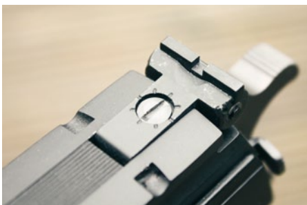
The rear sight is simple but adjustable.
