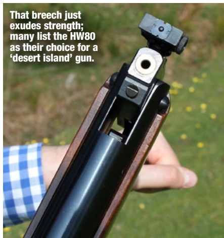
Rear sight offers differing blade options, which vary the sight picture.
