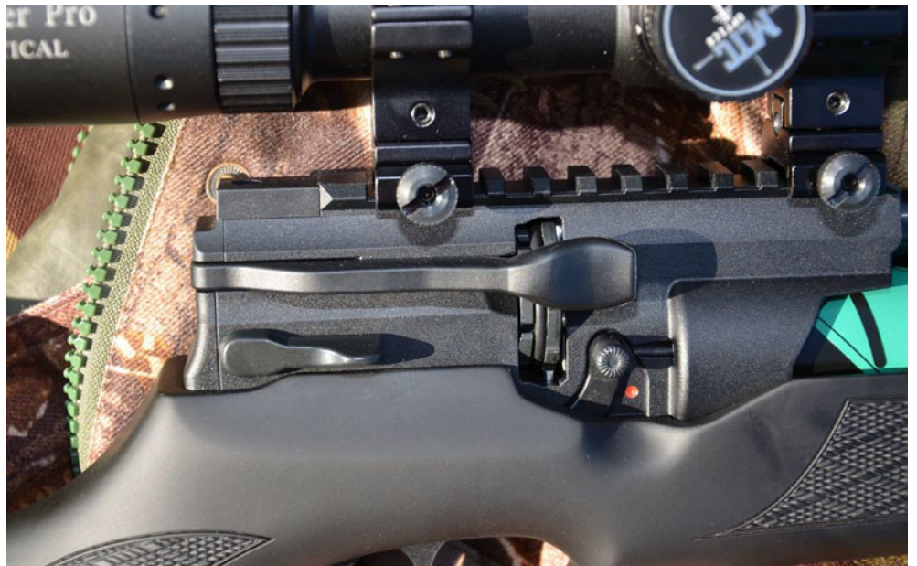
BELOW RIGHT: Fitting the mag' is a bit fiddly; note the retaining clip under the lever
