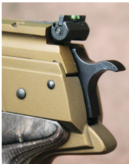
The faux hammer is the release catch for the action
