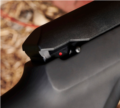
The resettable safety catch has a switch on both sides of the stock and can only be set when the gun is cocked
