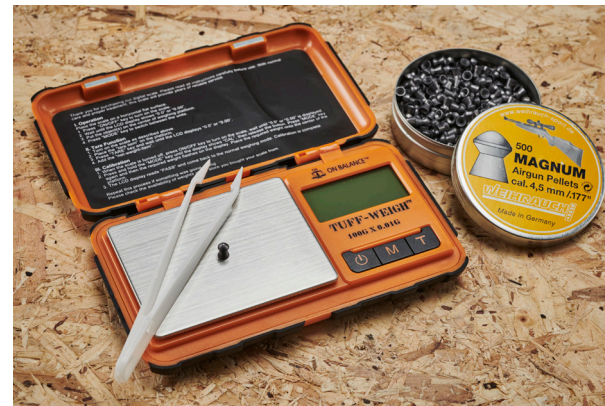
Putting a random sample of 50 pellets over the scales showed good consistency of weight, the average being 10.28 grains
