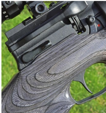
Action area. Sidelever, trigger, safety and mag' release lever. For me, the latter is on the wrong side.
