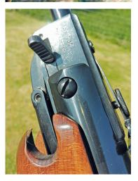
the catch hits against the receiver and something eventually addressed by Weihrauch as newer models have a roller inside to eliminate this noise. It's an excellent improvement because a rabbit's hearing does tend to pick up the sound of an early HW35 being cocked.
