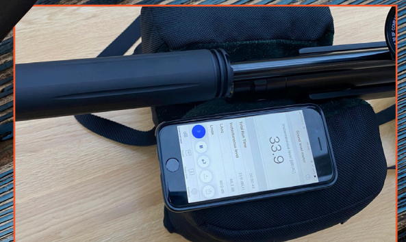
The Sound Level Meter app from the National Institute for Occupational Safety and Health is not only free, but produces reliable results as well
