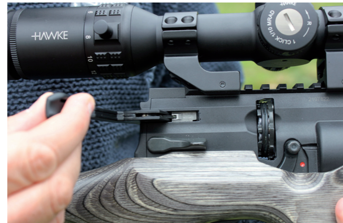
To remove the magazine draw back the cocking lever.
