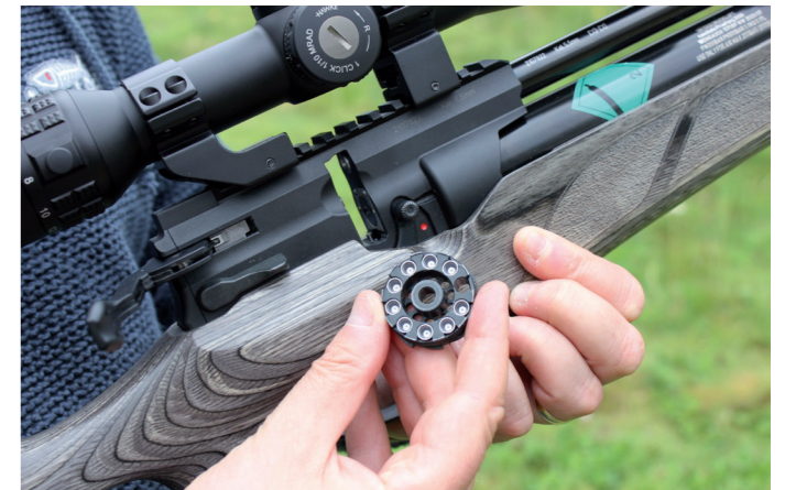
Ten-shot magazine, no moving parts, so nothing to fail, and you get two.
