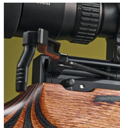
The safety catch is sensibly located well away from the trigger, but can only be applied once the rifle's been cocked
