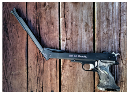
...while here it's been cocked to the high-power setting, with Phil getting up to 5.75 ft-lb from the test gun
