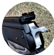
The fibre optic inserts on the precision open sights work well
