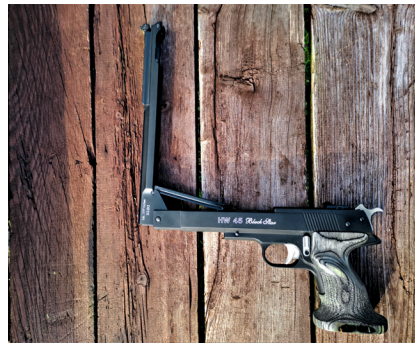
This pistol offers two power settings, and here the action has been cocked to the low-power setting...
