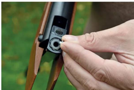
Each pellet is loaded into the breech as a single shot.
