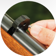
The pop-up loading gate may be quirky these days, but does mean the HW 57 offers the peace of mind of a fixed-barrel springer with the ease of loading of a break-barrel
