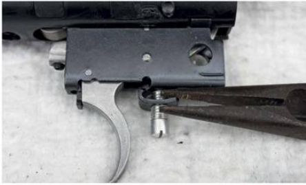
straighten out the bracket before removing the adjuster screw.
