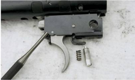
Drift out the trigger pin to remove the blade. Note the adjuster screw and its tensioning spring.
