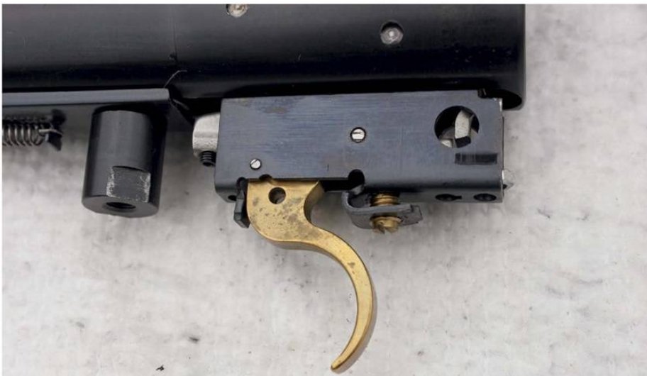
With the old blade out, insert the new blade, drift the pin back, and replace the tensioning spring before using the new adjusting screw.
