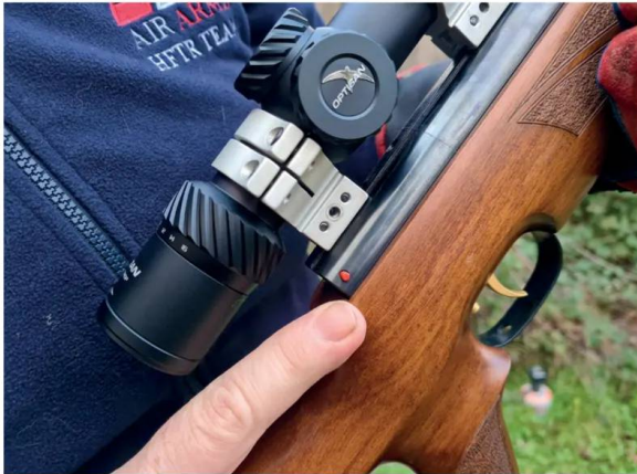
ABOVE LEFT: The simple safety catch gives a positive click and works well with the internal bear trap
