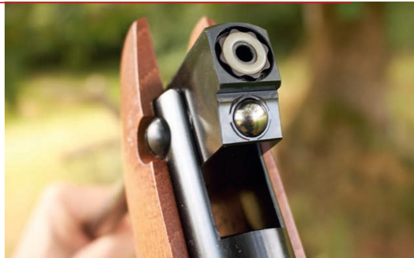
Ball detent takes the place of a chisel tip
